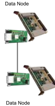
Figure 20: two node connection with XMC adapter
