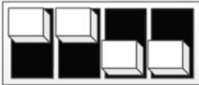
Illustration 6: SW1 – SWMODE - Default setting
