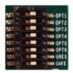
Figure 1: DIP Switch shows the DIP switch for the adapter card. It is used to select the operational mode. Please leave all undocumented DIP switches in the default position. Table 4: DIP Switch settings shows all the various DIP switch NTB settings for the adapter card.
