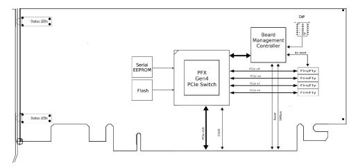
**Figure 3: Adapter card simplified schematics**
